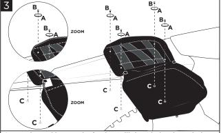
Center the tool bag on the fender. Drill the 4 holes through the fabric and the plastic. Fasten the 4 screws with the washers and nuts provided in the mounting kit.
