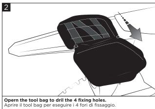
Opern the tool bag to dril the 4 fixing holes.
